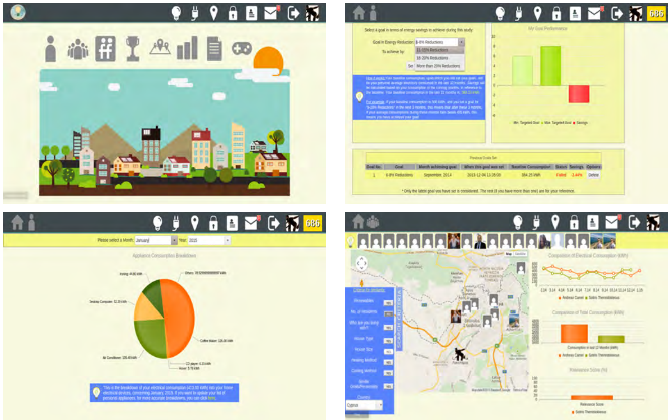
-Figure 3- Snapshots of Social Electricity: Main menu (top-left); Setting goals for energy savings (top-right); Detailed breakdown of overall consumption per electrical appliance (bottom-left); Comparison of production/consumption with similar users (bottom-right). (result of the project "Social Electricity Online Platform (SEOP), EU FP7-LLP-1-2013")
