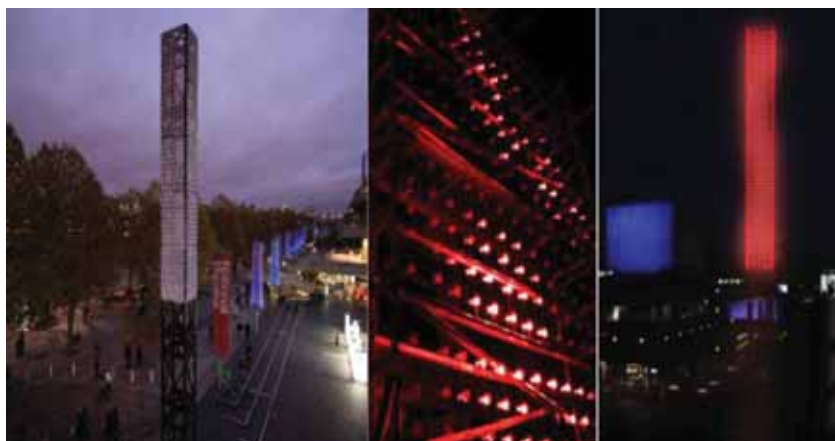
Aeolian toren South Bank London, wind aangedreven LED verlichting [9].
