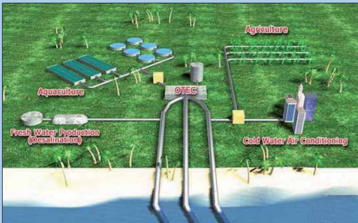
- Figuur 8 - OTEC plant on shore
